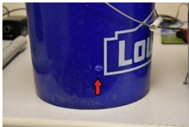
Figure 3 – Reservoir bucket with overflow hole
